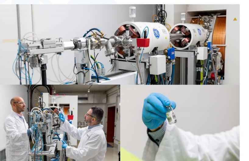
MITRU is home to **South Australia's only cyclotron** - a particle accelerator producing radioactive isotopes for use in medical imaging, treatment and research.
